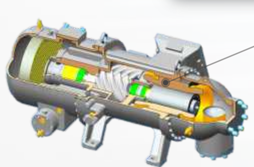
强制冷却结构示意图 Forced Cooling Structure Diagram ( 图6 ) (Fig.6)
